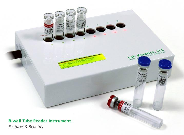
**Lab Kinetics Incubating 8-well Tube Reader** *Incubating (37°C)* tube reader capable of reading at 405 nm and 495 nm with a range of at least 0 - 1.0 Absorbance Units and accommodates vials of 12 mm diameter
